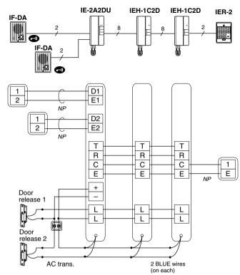
Run door release wires in a separate jacketed cable from the audio wires.
