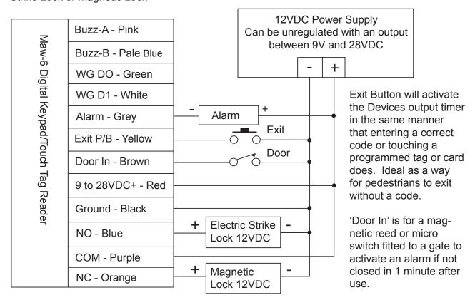
For 12V Automatic Gate Operator or 240V Operator with 12VDC output for accessories.
